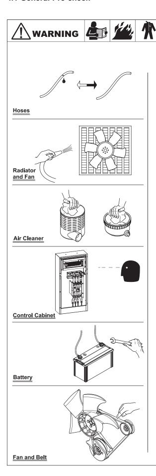
Before starting the genset, check each item below to make sure that the machine can be started up properly and reduce any possible problems.
